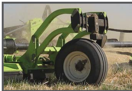
- Adjustable front castor wheels -
