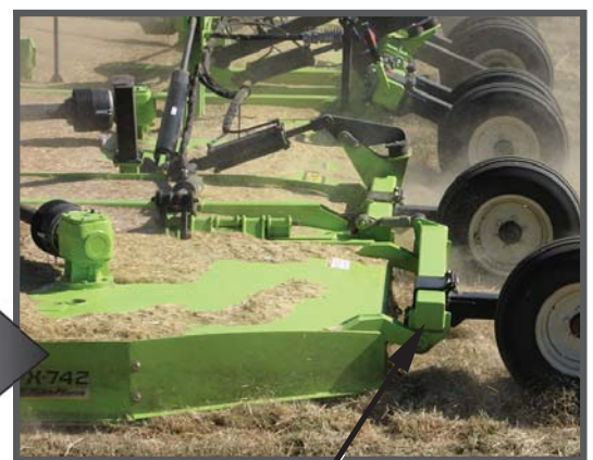
- Adjustable wheel standards for row crop spacing -
