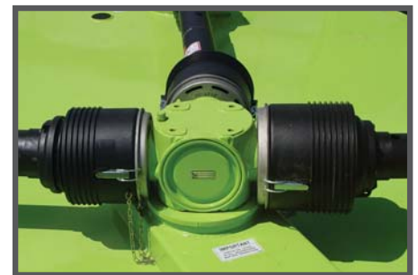
- 180hp divider box allows for unique driveline layout -
